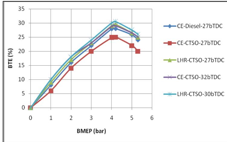
**Figure 4: Variation of BTE with BMEP in Both Versions of the Engine at Recommended and Optimized Injection Timings with CTSO Operation at an Injection Pressure of 190 Bar**
